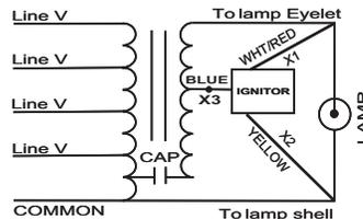
CW Autotransformer ballast
